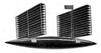
According to this present invention a number of these blades are placed one above the other in a frame, and two or more of these frames are attached to the upper part of a body which is propelled by apparatus not described or shown.
